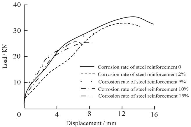
Figure 9: Curves of load-displacement (axial compression ratio 0.4).
