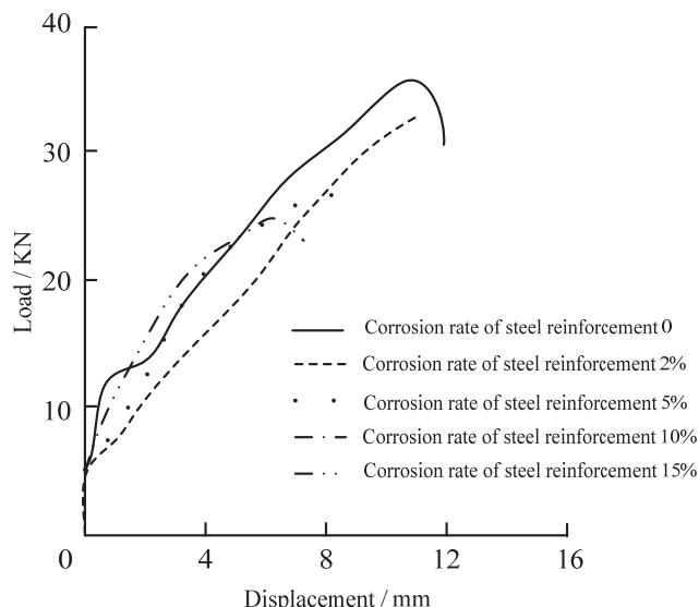
Figure 8: Curves of load-displacement (axial compression ratio 0.2).
