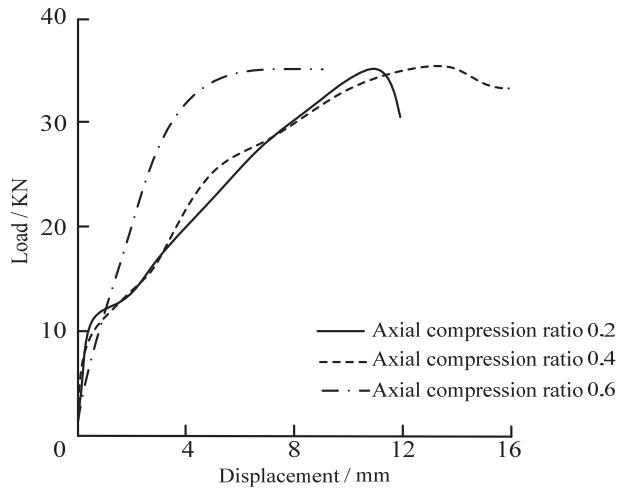
Figure 11: Curves of load-displacement (corrosion rate 0%).
