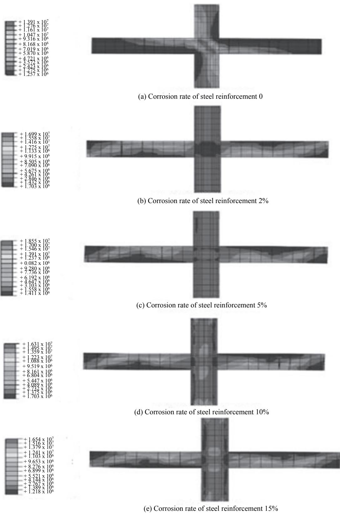
Figure 7: Nephogram of stress on joints of concrete.
