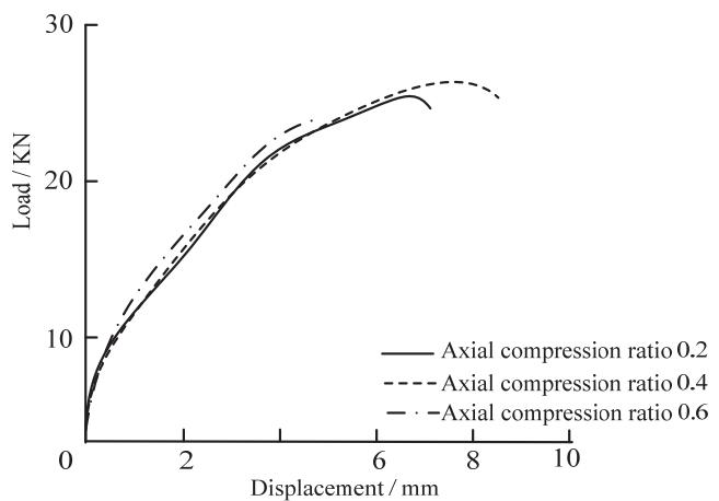
Figure 14: Curves of load-displacement (corrosion rate 10%).
