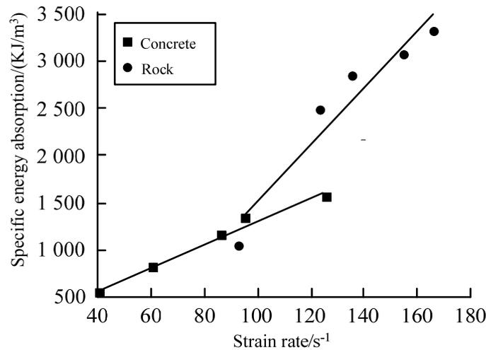
Figure 5: Correlation between specific energy absorption and strain rate.
