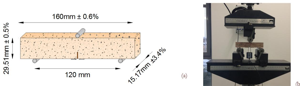
Figure 1: (a) Specimen geometry mean values and variations; (b) experimental set up of the Instron testing machine.
