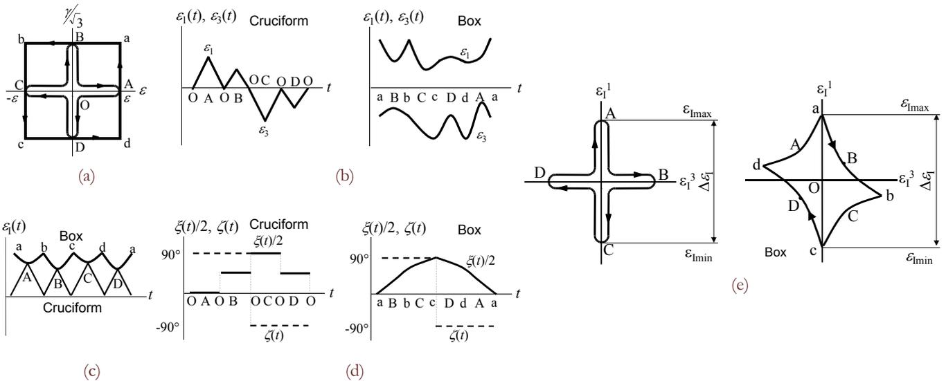
Figure 5: Variations of  $\varepsilon_1(t)$ ,  $\varepsilon_3(t)$  and  $\xi(t)/2$  in non-proportional straining: (a) Strain paths on  $\varepsilon-\gamma/\sqrt{3}$  plot, (b) Variation of  $\varepsilon_1(t)$ , (c) Variation of  $\varepsilon_1(t)$ , (d) Variation of  $\xi(t)$  and  $\zeta(t)$ , (e) Strain paths on polar figure.
