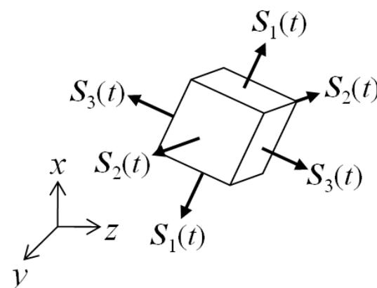
Figure 1: Principal stress and strain in xyz coordinates.
