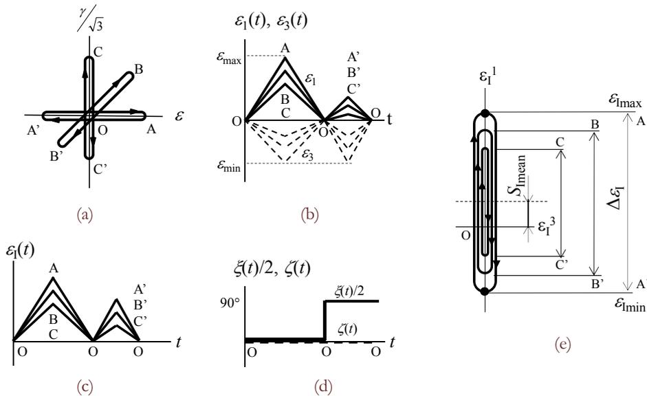
Figure 4: Variations of  $\varepsilon_1(t)$ ,  $\varepsilon_3(t)$  and  $\zeta(t)/2$  in proportional straining: (a) Strain paths on  $\varepsilon - \gamma/\sqrt{3}$  plot, (b) Variation of  $\varepsilon_1(t)$ , (c) Variation of  $\varepsilon_1(t)$ , (d) Variation of  $\zeta(t)$  and  $\zeta(t)$ , (e) Strain paths on polar figure.
