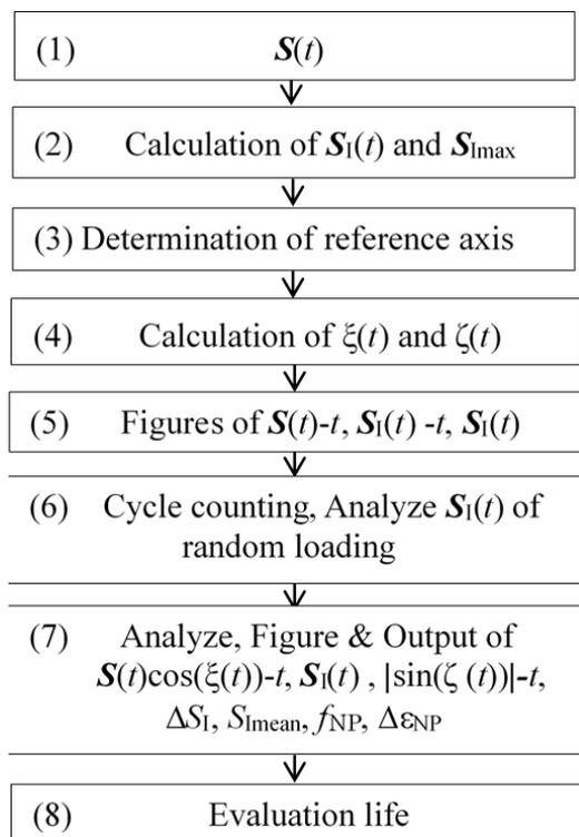
Figure 11: Calculation flow in the program.
