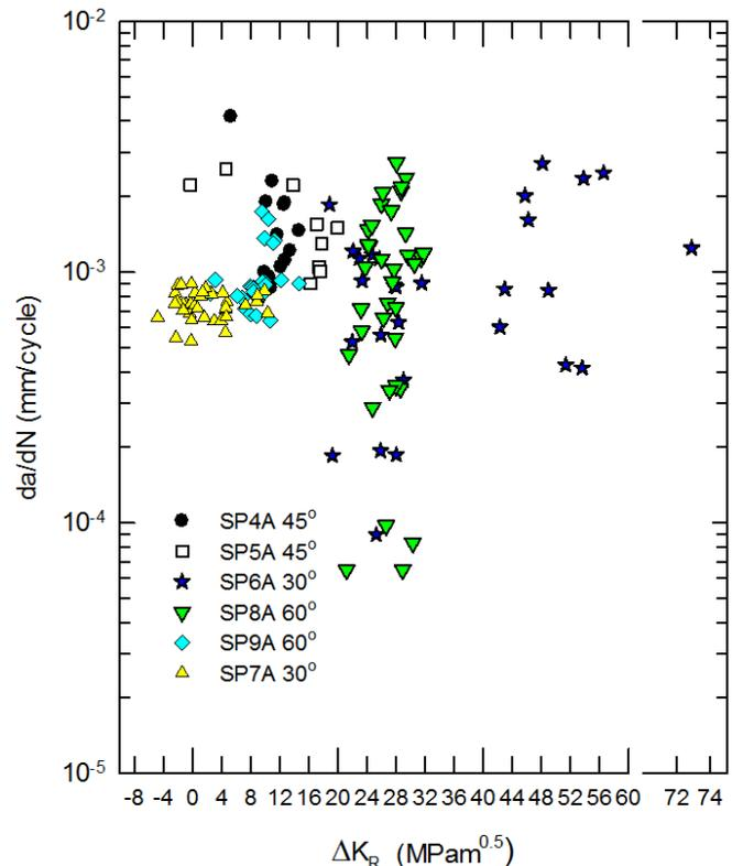
Figure 5: Fatigue crack growth rate data for all inclined crack specimens plotted against  $K_R$ .
