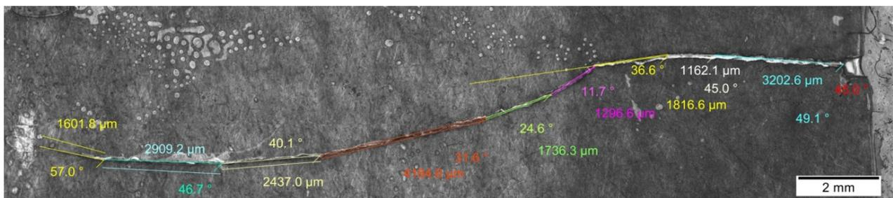
Figure 3: Illustration of the varying crack path angle on an acetate surface replica for specimen SP5A with an initial 45° slit. The arrow indicates the direction of the applied load during the crack growth under biaxial stresses.
