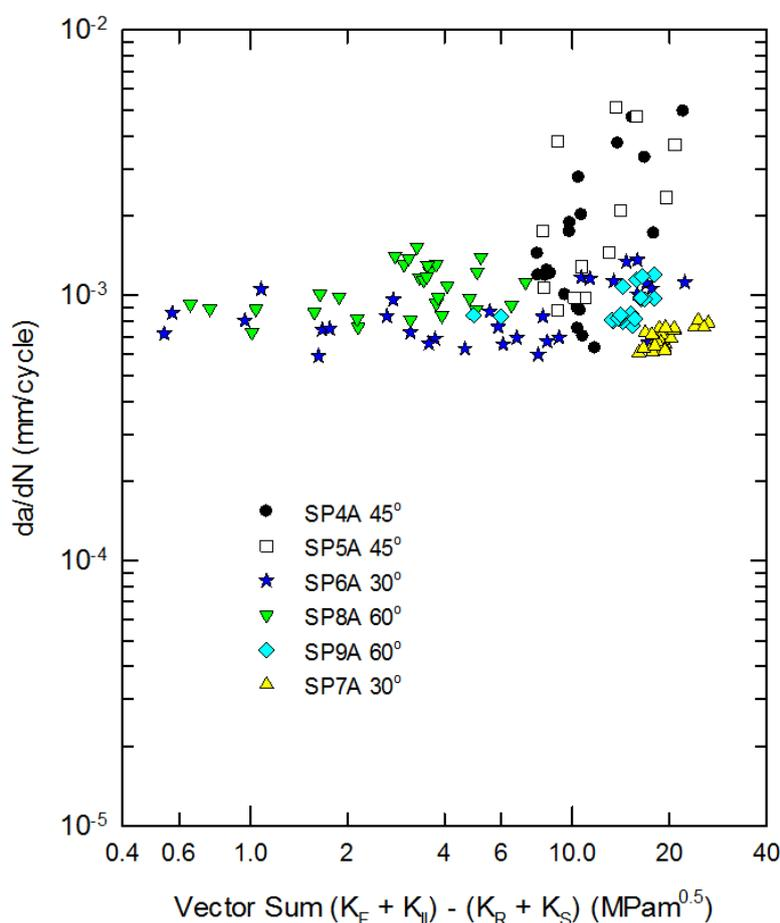
Figure 6: Reduction in scatter obtained by using the net vector sum driving force, expressed as a stress intensity factor.
