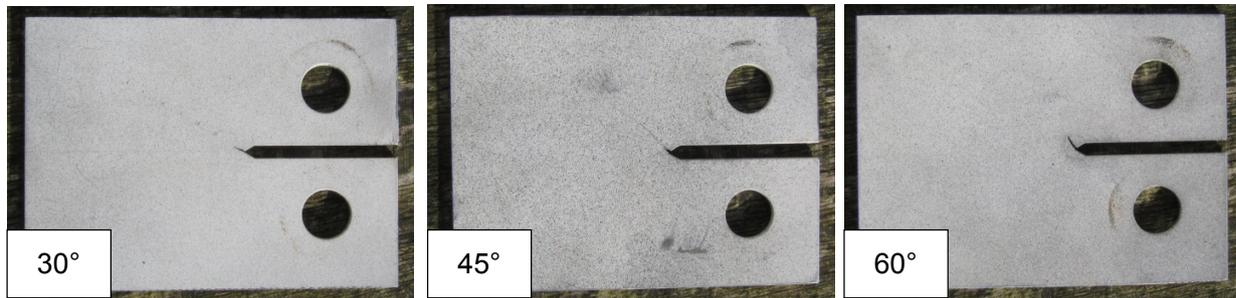
Figure 1: Typical aluminium CT specimens used in this work. In these specimens the initial inclined slit has been extended by fatigue crack growth.
