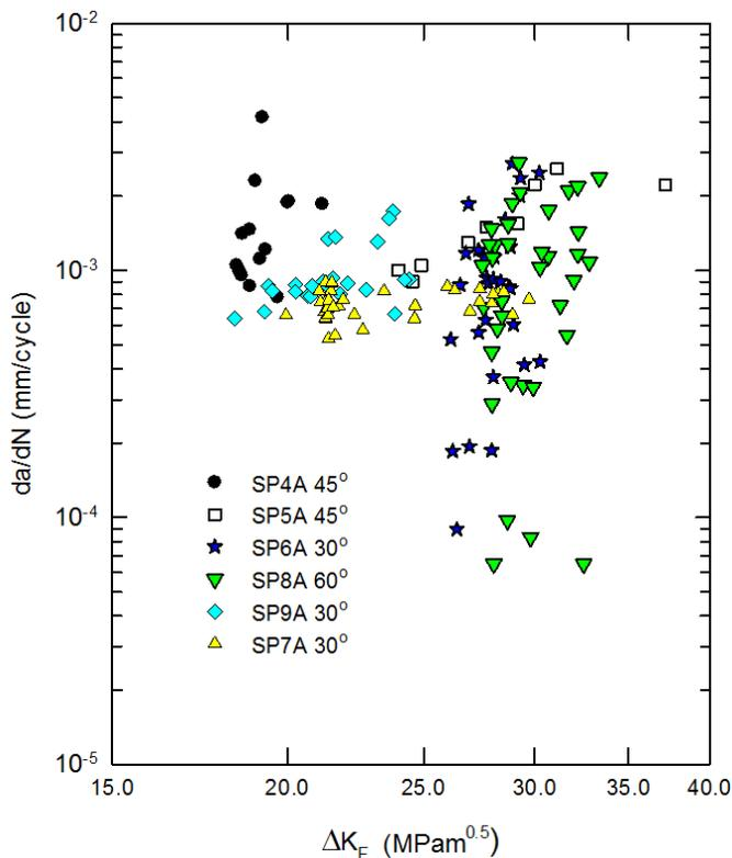
Figure 4: Fatigue crack growth rate data for all inclined crack specimens plotted against  $K_F$ .
