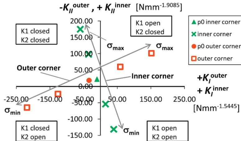
Figure 5: Diagram of  $K_{II}$  versus  $K_I$  showing the implications of Williams' solution for contact behaviour [11].
