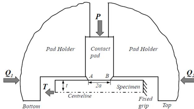
Figure 2: Idealised diagram of the pad-on-dogbone test rig [5].
