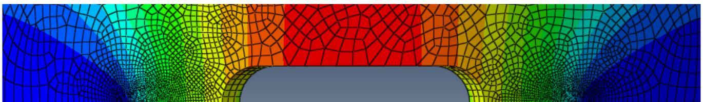
Figure 26: Example for the calculation of stress intensity factors, here vertical displacements of a 6mm crack, compare with Fig. 8, red color means displacements larger than  $29\mu\text{m}$ .
