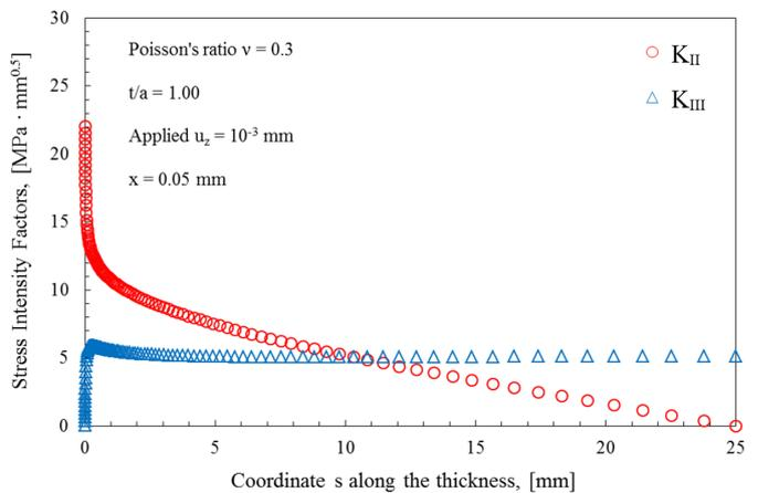
Figure 7: Through thickness distribution of  $K_{II}$  and  $K_{III}$  for:  $t/a = 1$ ,  $x = 0.05$  mm.
