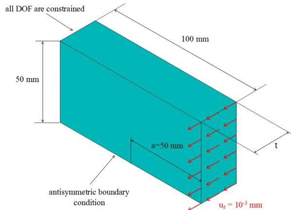
Figure 2: Plate geometry.
