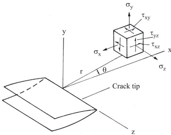
Figure 1: Notation for crack tip stress field.
