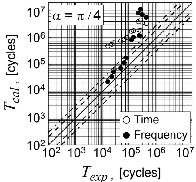
Figure 5: Comparison between experimental and theoretical fatigue lives ( $\alpha = \pi/4$ ), the latter determined by employing: the frequency domain criterion here proposed (see solid symbols) and the time domain criterion reported in Ref. [4] (see hollow symbols).
