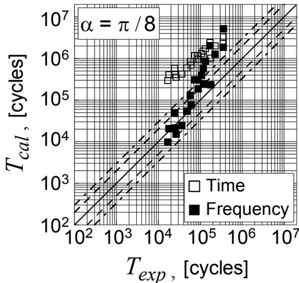
Figure 4: Comparison between experimental and theoretical fatigue lives ( $\alpha = \pi/8$ ), the latter determined by employing: the frequency domain criterion here proposed (see solid symbols) and the time domain criterion reported in Ref. [4] (see hollow symbols).
