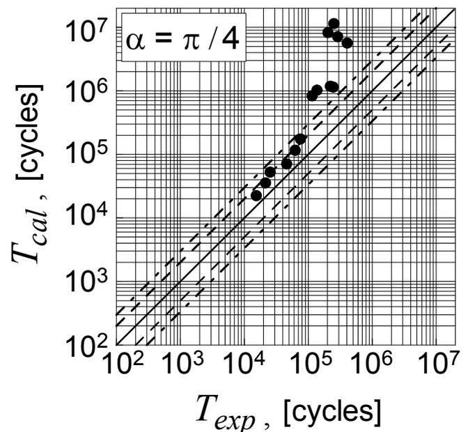
Figure 3: Comparison between experimental and theoretical fatigue lives ( $\alpha = \pi / 4$ ).
