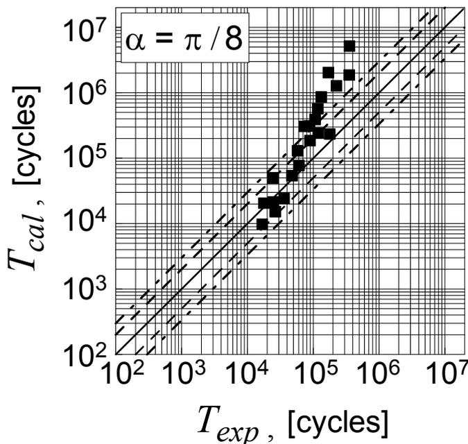
Figure 2: Comparison between experimental and theoretical fatigue lives ( $\alpha = \pi / 8$ ).
