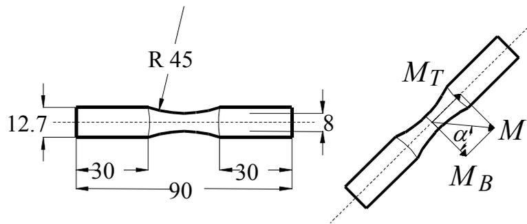
Figure 1: Fatigue tests on round specimens (10HNAP steel): torsion and bending.
