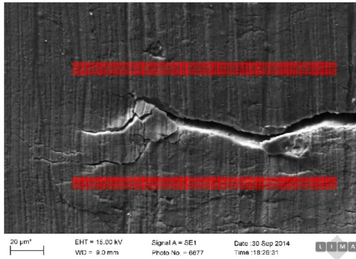
Figure 4: Typical image collected from the experiment at a load of 1:25 kN. Sets of points are selected on either side of the crack to measure displacements.
