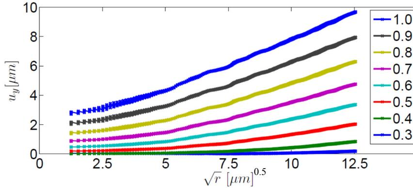
Figure 7: Variations of relative displacement ( $u_y$ ) with distance from the crack tip ( $r$ ) at eight different values of load ( $P/P_{max}$ ) during the loading phase of a single cycle.
