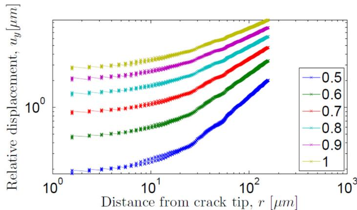
Figure 6: Variation of relative displacement ( $u_y$ ) with distance from the crack tip ( $r$ ) at five different values of load ( $P/P_{\text{max}}$ ) during the loading phase of a loading cycle.
