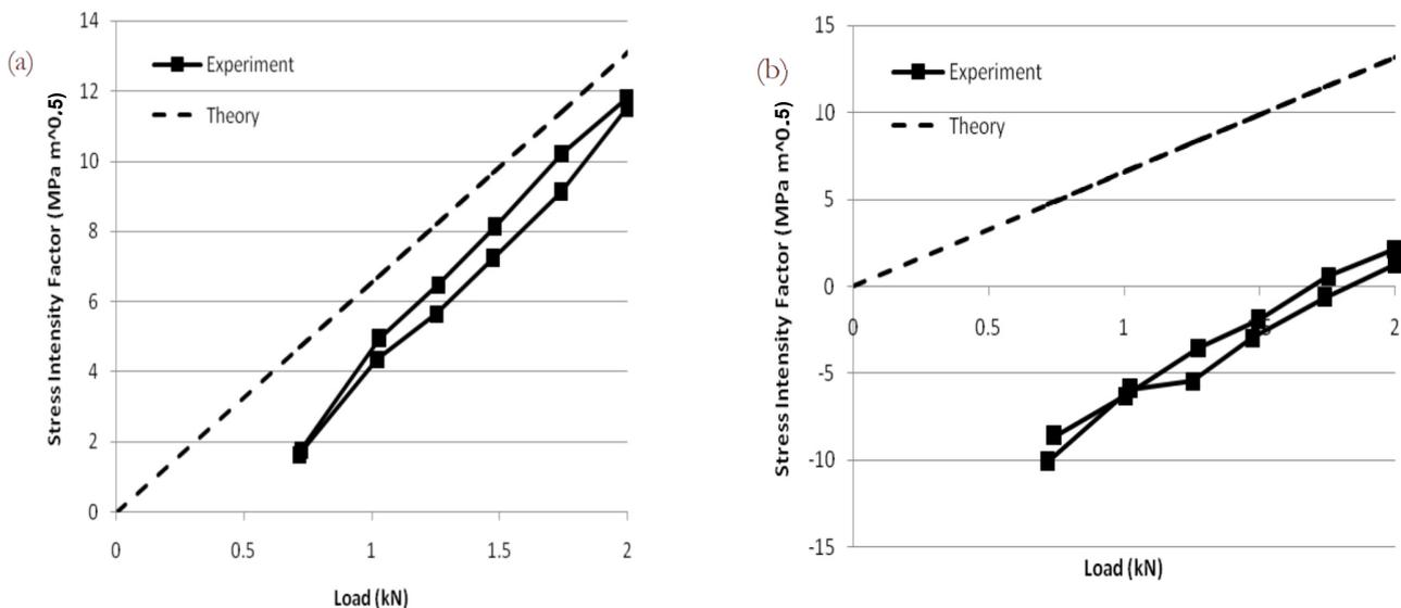
Figure 1: Variation of measured stress intensity factor with load for specimen CTF6 [4] (a) After constant amplitude loading and (b) Immediately after an overload.
