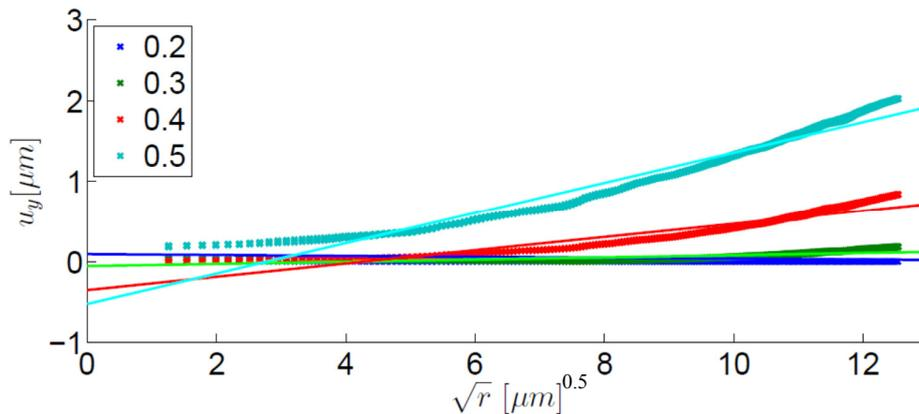
Figure 10: Variations of relative displacement ( $u_y$ ) with distance from the crack tip ( $r$ ) at four different values of load ( $P/P_{max}$ ) during the initial loading phase of a single cycle. A line of best fit produced with a least squares method is included for each load in the matching colour.
