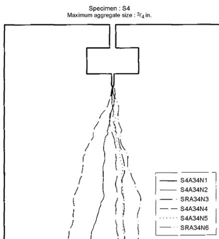
Figure 3: Experimentally observed crack trajectories in concrete specimens.
