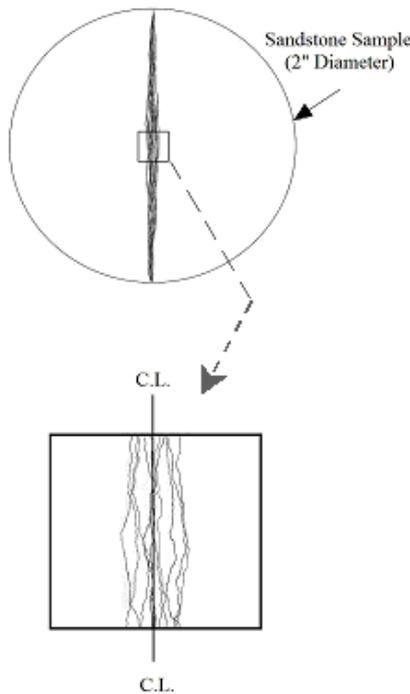
Figure 1: Experimentally observed crack trajectories in sandstone discs.
