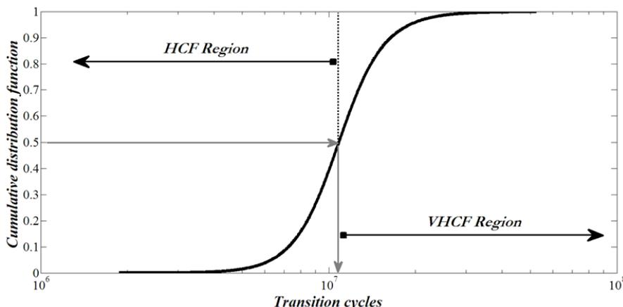
Figure 4: Statistical distribution of the transition life together with the probable fatigue regions.
