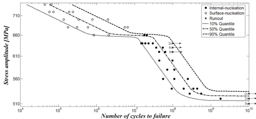
Figure 3: Quantile S-N curves.
