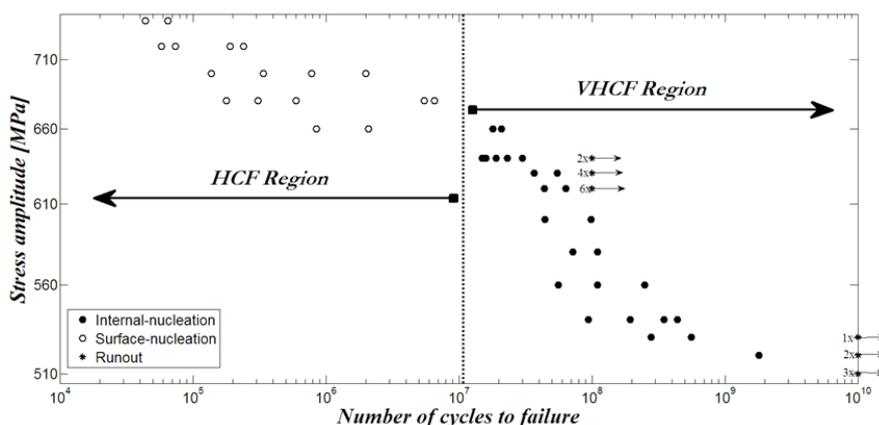
Figure 5: Experimental data and probable fatigue regions as discriminated by the median value of the transition life.
