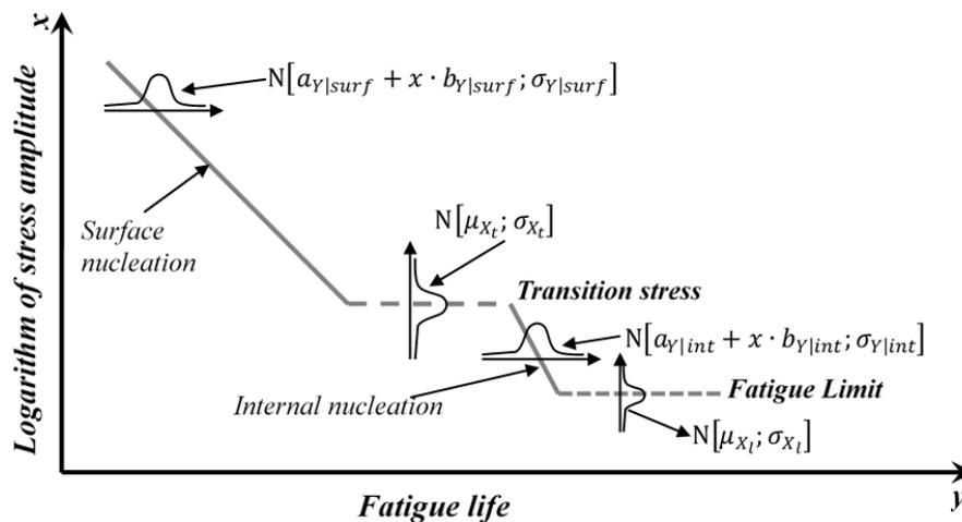
Figure 1: Schematic of a statistical Duplex S-N curve with fatigue limit.
