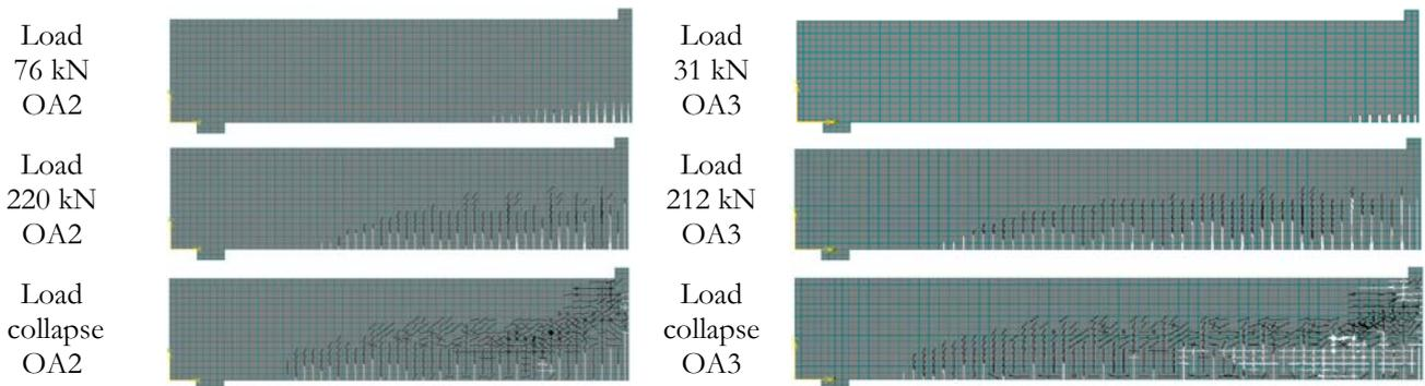
Figure 6: Failure in a beam. OA2 (left) and OA3 (right).
