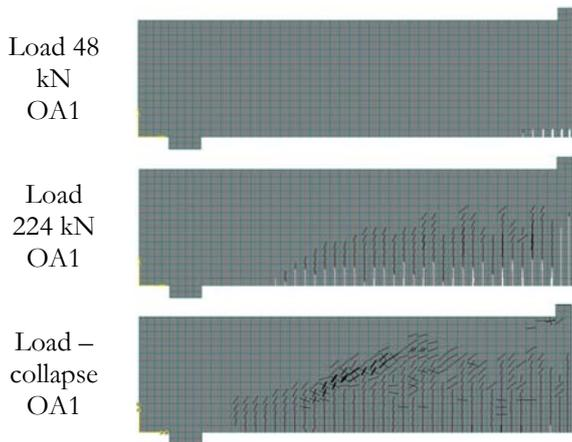
Figure 4: Failure in a beam, OA1.
