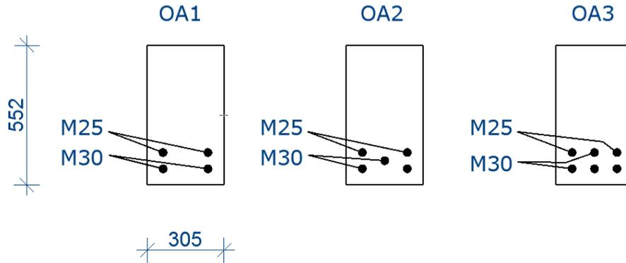
Figure 2: Cross-section of the beams.
