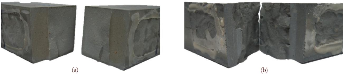
Figure 8: Fracture surface of cement composite samples (a) Cement (b) Cement with 0.08wt% carbonized hemp hurds
