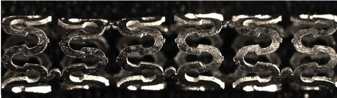
Figure 8: Optical microscopy image of the AZ31 after chemical etching.
