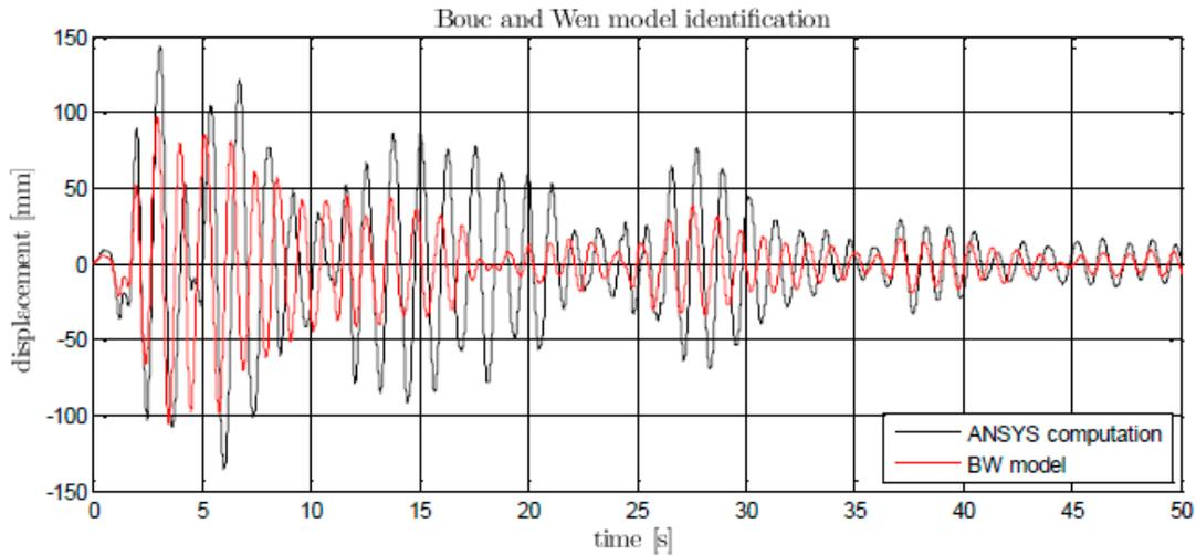
Figure 4: Displacement time history: comparison between BW identified model and ANSYS results (2<sup>nd</sup> attempt).
