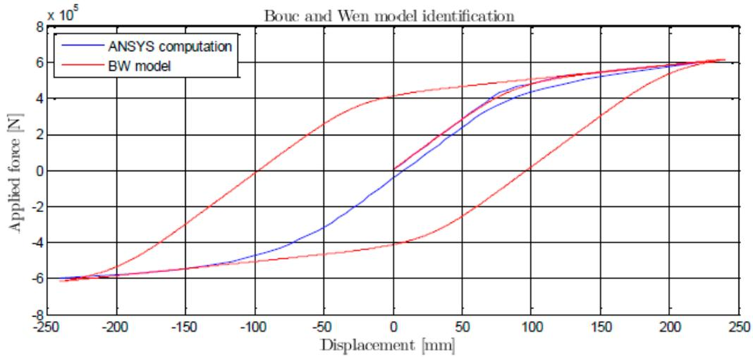
Figure 2: Comparison of the identified BW model with the ANSYS results (1<sup>st</sup> attempt).
