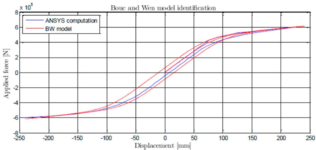
Figure 3: Comparison of the identified BW model with the ANSYS results (2<sup>nd</sup> attempt).
