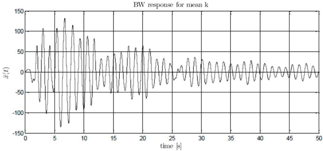
Figure 9: Response  $\bar{x}(t)$  evaluated for  $\bar{k} = E[k]$ .
