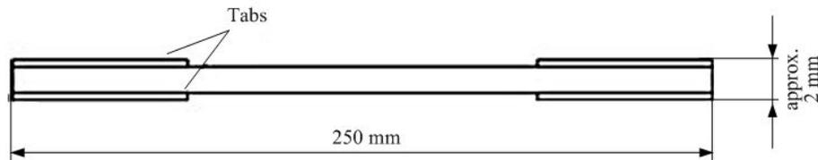
Figure 3: Side view of the tensile test specimens with tabs according to German standard DIN EN 2747 [7].
