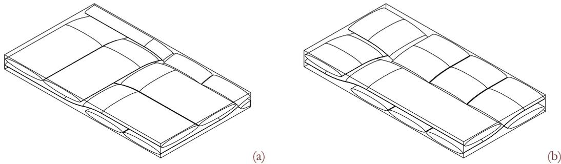
Figure 5: 3D models of the RVE. (a) Twill weave 2/2; (b) Twill weave 1/3.
