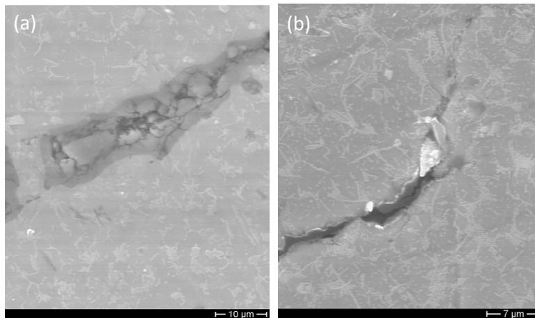
Figure 6: SEM micrographs showing two details of cracks that propagated in the Alloy “A” casting
