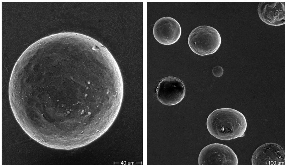
Figure 3: SEM micrographs showing gas porosity on the external surface of Alloy “C” specimen.
