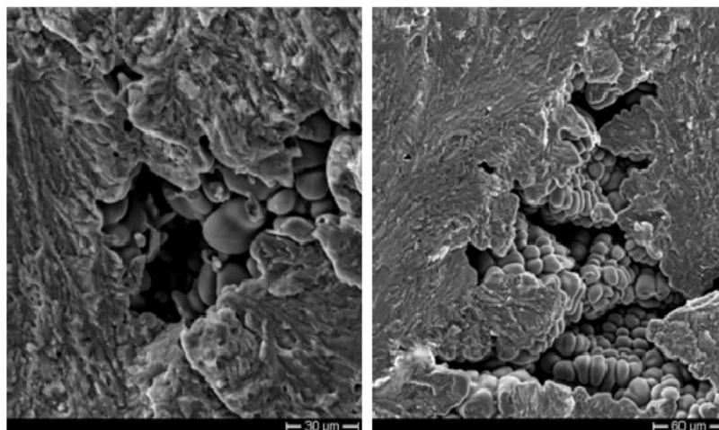
Figure 5: Shrinkage cavities found in the Alloy “P”.
