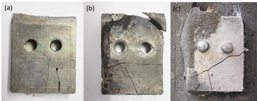
**Figure 1:** Macrograph showing three fractured specimens (34x40x10 mm<sup>3</sup>). Specimen shown in macrograph (a) was cast under vacuum while specimens in macrographs (b) and (c) were cast under argon atmosphere.
