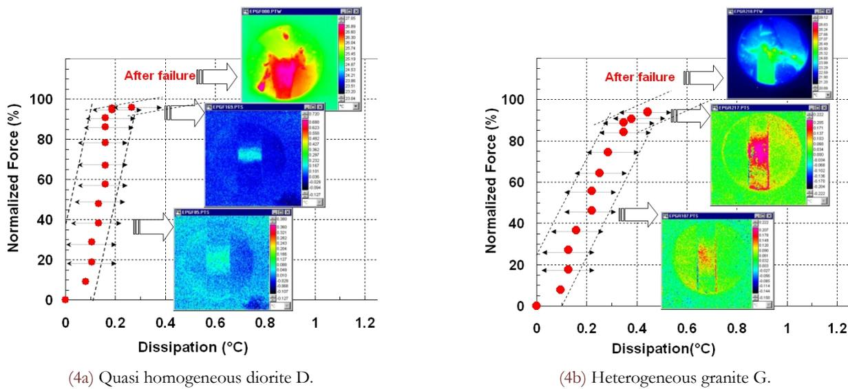
Figure 4: Different stages of heat dissipation describing the process of the damage extent in the granite specimen (characterized by its compressive strength  $R_c$ ). Graphical determination of the threshold of acceptable damage TAD of tested materials subject to unconfined loading up to failure.
