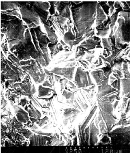
Figure 9: Fracture surface of implant failed in service.
