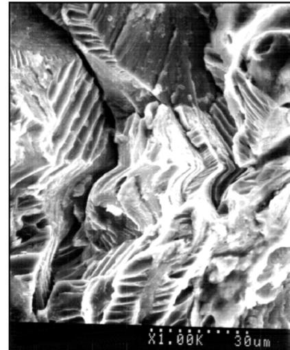
Figure 10: Fracture surface of implant failed in service.
