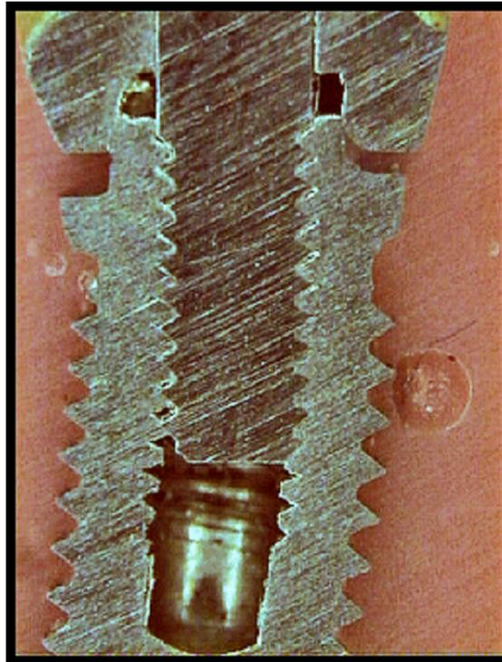
Figure 11: Screw implant, deformed after the test.
