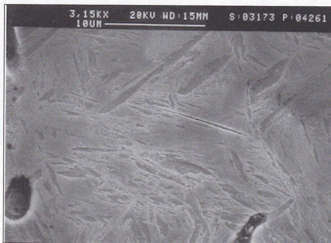
Figure 10: MSP 4 SEM micrograph: martensite with some islands of transforming austenite.
