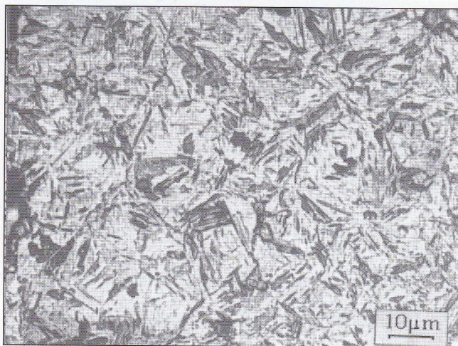
Figure 9: MSP 4 LOM-micrograph - Thin martensite associated with transforming austenite.
