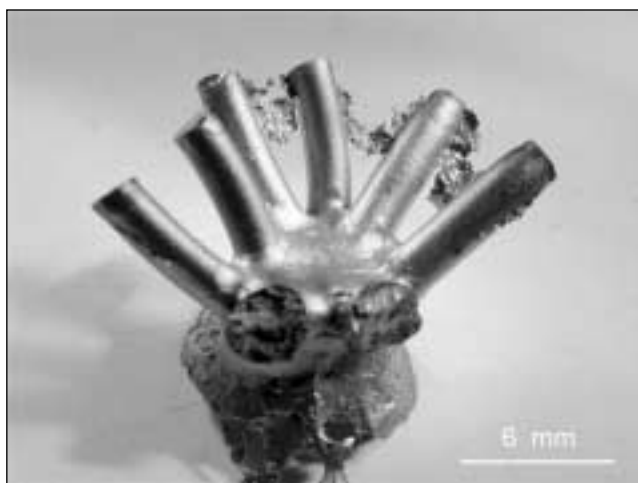
Fig. 15 – Typical fins on a portion of the former sprue, due to the investment breaking during pre-heating of the dental casting mold.
