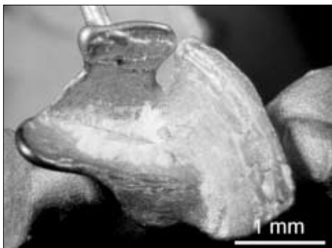
Fig. 14 – Incomplete device due to a too low casting temperature.
