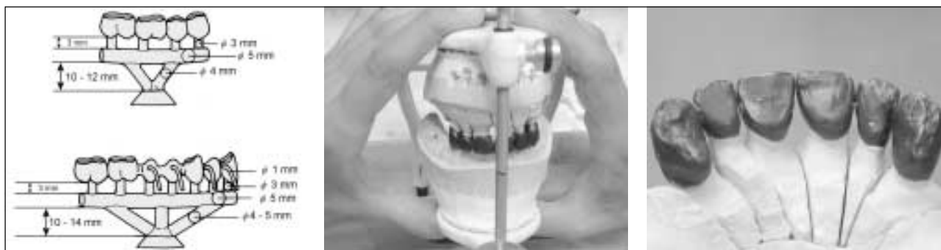
Fig. 1 – Figures show some steps of the wax pattern preparation. On the left some recommended sprue dimensions are given.
