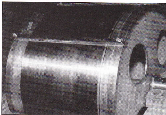
Fig. 1 - SCS6 fibres positioned onto a cylindrical substrate.
