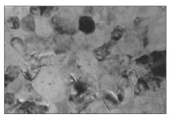
*Fig. 5 – Thin foil structure from the TiN/(Ti,Al,Si)N/TiN gradient coating deposited on the CER2 cermet.*
