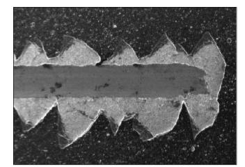
*Fig.* 8 – *Indenter trace with the maximum load on the TiN/(Ti,Al,Si)N/TiN gradient coating surface deposited onto the CER2 cermet.*
