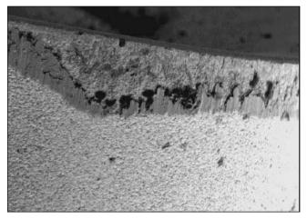
Fig. 11 – Flank wear nature of the CC1 type uncoated cemented carbides ( $f=0.1 \text{ mm/rev}, a_p=1 \text{ mm}, v_c=315 \text{ m/min}$ ).
