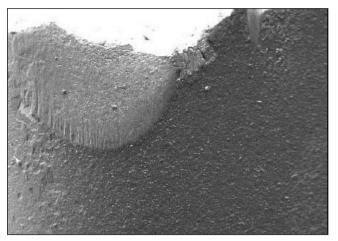
Fig. 10 – Flank wear nature of the CER2 type cermet with the TiN/(Ti,AI,Si)N/TiN coating (f=0.1 mm/rev,  $a_p=1$  mm,  $v_c=400$  m/min).
