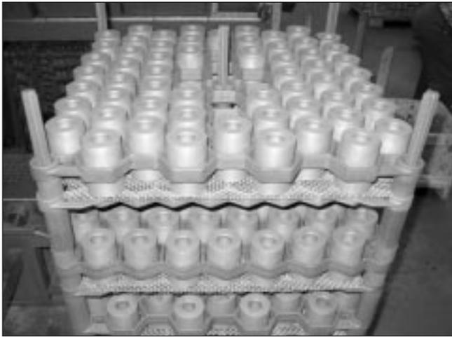
Fig. 10 – Load of 144 piston pins case-hardened to 1.0 to 1.5 mm.
