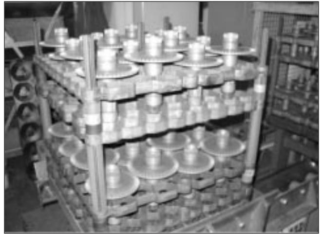
Fig. 12 – Case-hardened parts of a cvt-transmission.
