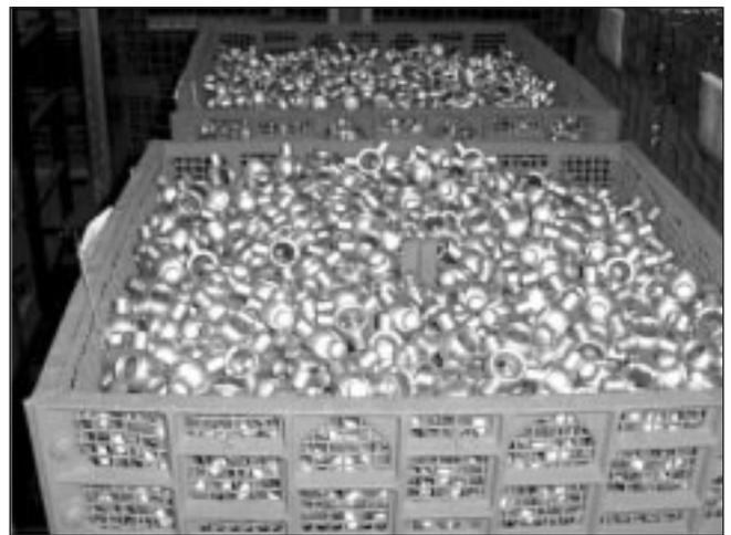
Fig. 13 – Loads of tripod forgings to be normalized.
