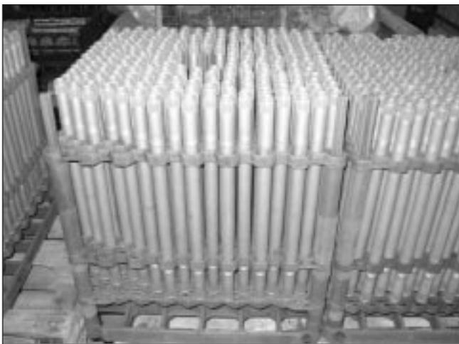
Fig. 11 – Load of 221 shafts case-hardened to 0.8 to 1.1 mm.
