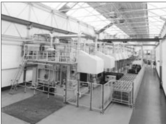
pusher furnace used for isothermal annealing. It consists of a high-temperature furnace running at 900°C, a rapid gas cool station bringing the loads down to 650°C, an isothermal annealing furnace (650°C) and a cooling zone. The total capacity of this pusher annealing furnace line is approx. 825 kg/h. In figure 6 an example of a soft annealing or re-crystallization pusher furnace line is shown with a heating section (to
