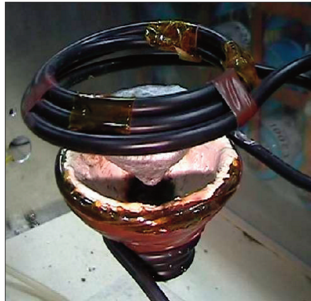
FIG. 12 Levitating molten Al inside the experimental crucible-less system.
