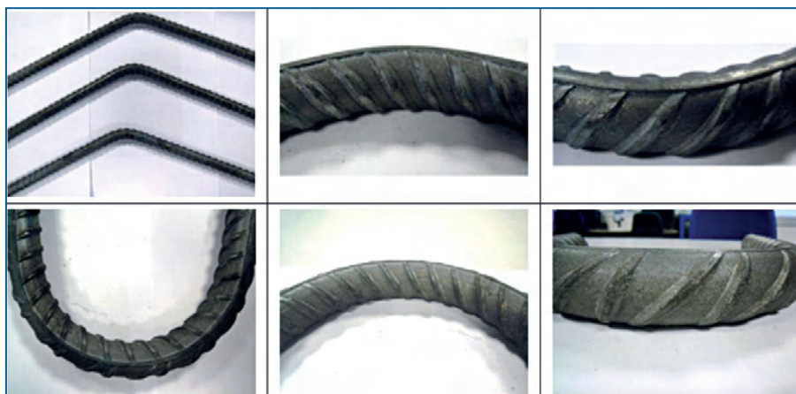
Fig. 8 – Bend tests done on samples of high-tensile rebar heat-treated in line.
