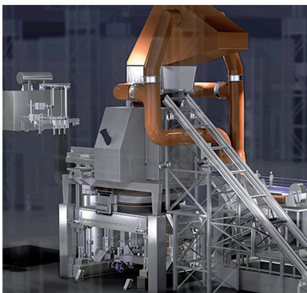
Fig. 7 - Simetal EAF QUANTUM Furnace® represents the latest evolution of the shaft furnace with the scrap basket, through which the hot fumes pass, located above the EAF.
