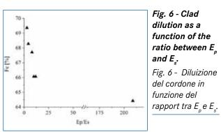
$E_s$ . Since  $E_{eff}$  is observed to increase with  $E_p$  and  $E_s$  has a minor effect, it may be concluded that the processing conditions that improve the energetic efficiency tend to reduce dilution of the clad.
