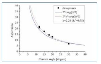
Fig. 8 - Aspect ratio as a function of the contact angle
