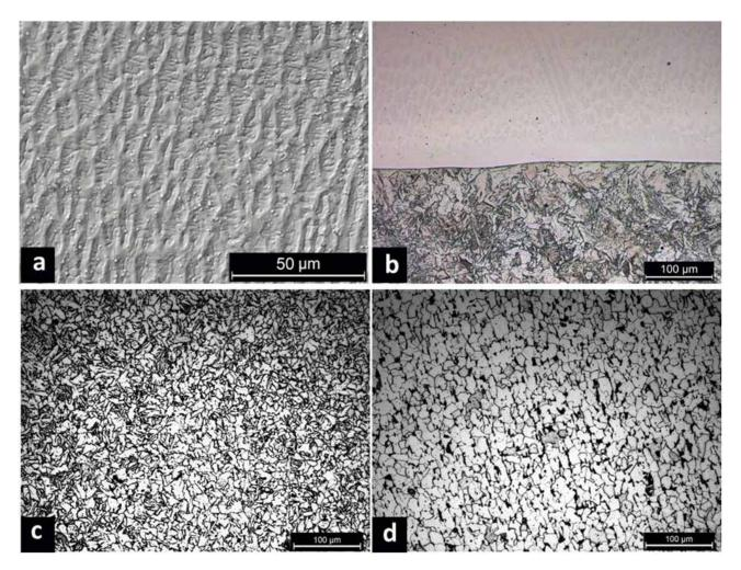
Fig. 2 - Cellular solidification structure of the clad (2a), microstructure at the interface (2b) and coarse bainitic (close to interface) and pearlitic/ferritic microstructure (close to unaffected substrate) HAZ (2c and 2d) in clad 3.
