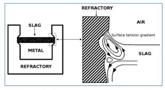
Fig. 4 - Mechanical interaction between the slag and the surrounding refractory lining due to the effect of the surface tension [9].
