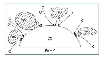
Fig. 5 - Scheme of CO bubble formation in slag through the reaction among iron oxide droplets, carbon and oxygen [12].
