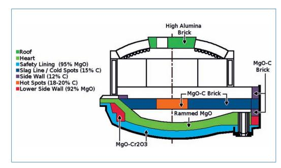
Fig. 1 - Schematic cross section of an electric arc furnace indicating the typical refractories employed.
