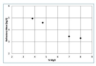
Fig. 9 - Specific refractory wear as a function of MgO weight concentration in slag.
