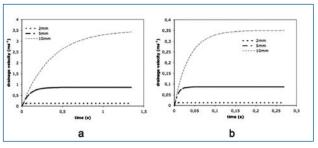
Fig. 8 - Trend of drainage velocity as a function of bubble radius and the viscosity (a) 43·10<sup>-6</sup> Pa·s (b) 500·10<sup>-6</sup> Pa·s [13].
