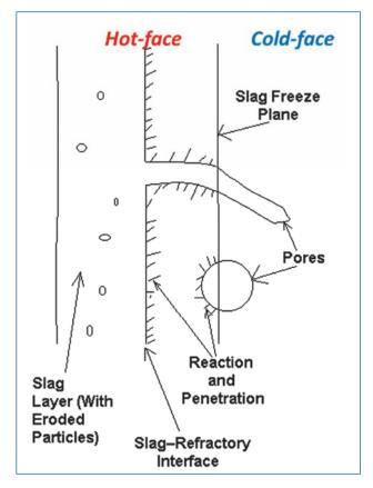
Fig. 2 - Cross section of the slag-refractory interfacial area [8].
