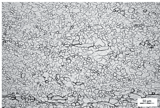
Fig. 5 - Microstructure after TRC, rough rolling and intermediate annealing.
