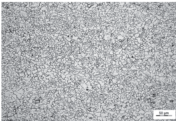
Fig. 6 - Microstructure after intermediate annealing and finish rolling.
