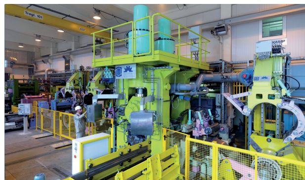
Fig. 2 - TRC- and Strip Rolling process for magnesium strip at the Institute of Metal Forming.
