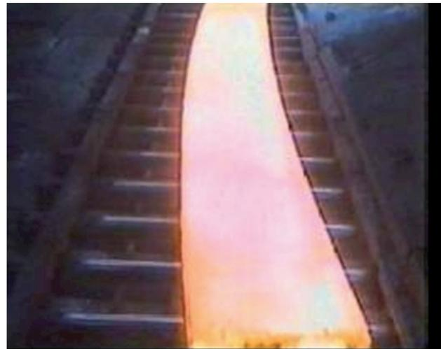
**Fig. 1- Example of a bar in the rougher mill with severe (head) camber.**
