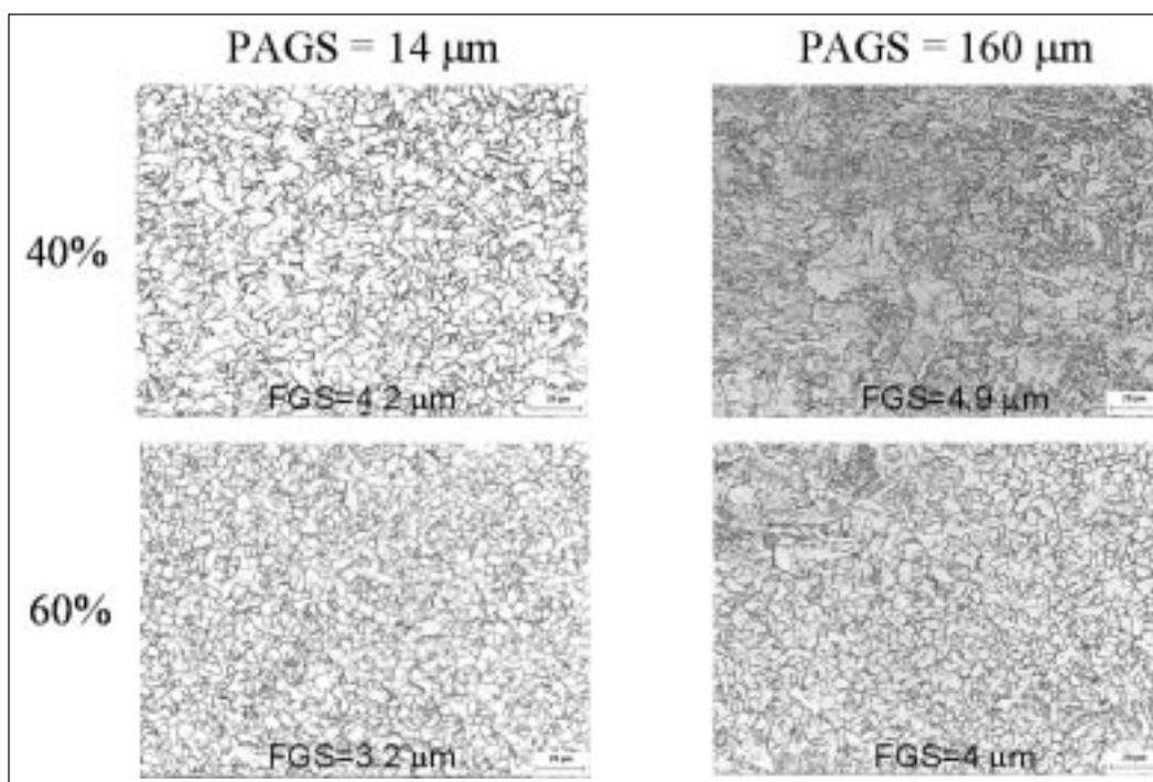
In Fig. 2 the microstructures of sample B are shown.
