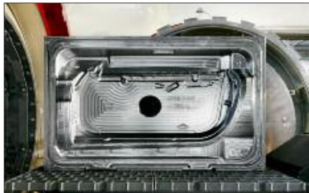
**FIG. 9** *Die insert for a passenger car door, 3.820 kg.*
