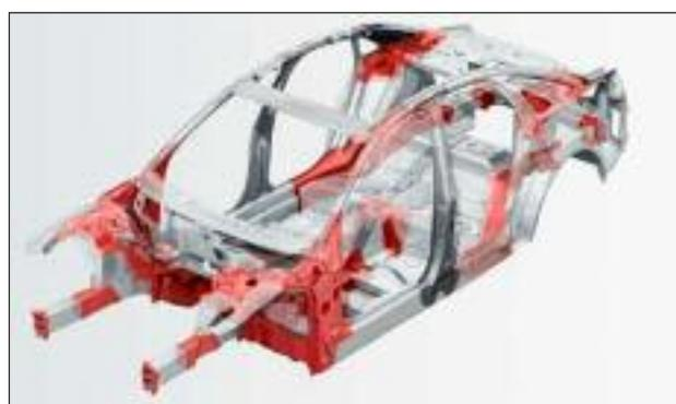
**FIG. 1** Cast aluminium structural components (red) in the auto body of the AUDI A 8 [4].
