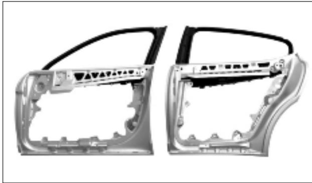
**FIG. 2** Door and window frames for a German sports car (Photo: Georg Fischer AG).
