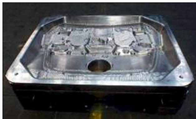
**FIG. 10** *Die insert for a hatchback support frame, 1.350 mm x 1.720 mm x 440 mm, 5.440 kg.*
