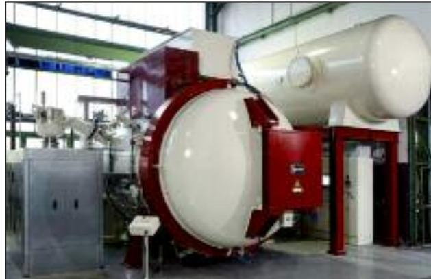
**FIG. 8** *New vacuum hardening furnace Ipsen Turbo Treater ST6672 at Kind & Co.*
