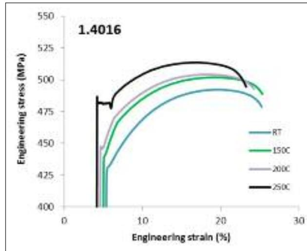
**FIG. 5** Stress-strain curves for 1.4016 aged at different temperatures. Curves have been displaced by 0.40% along the abscissa to avoid crowding.
