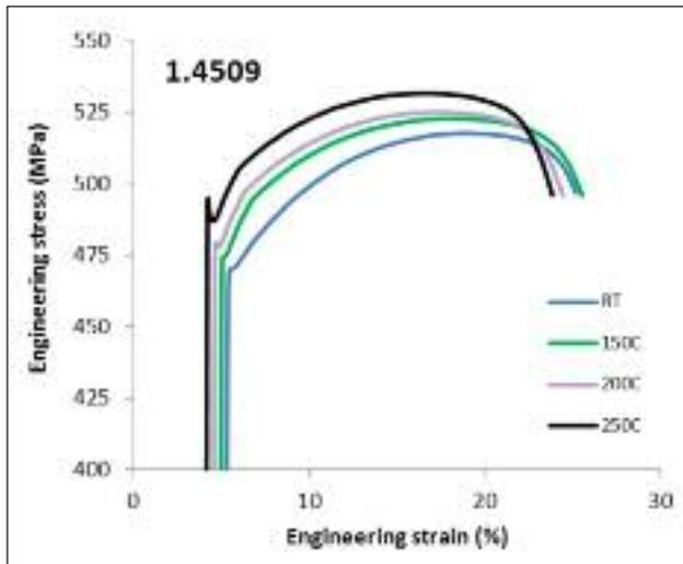
**FIG. 3** Stress-strain curves for 1.4509 aged at different temperatures. Curves have been displaced by 0.40% along the abscissa to avoid crowding.
