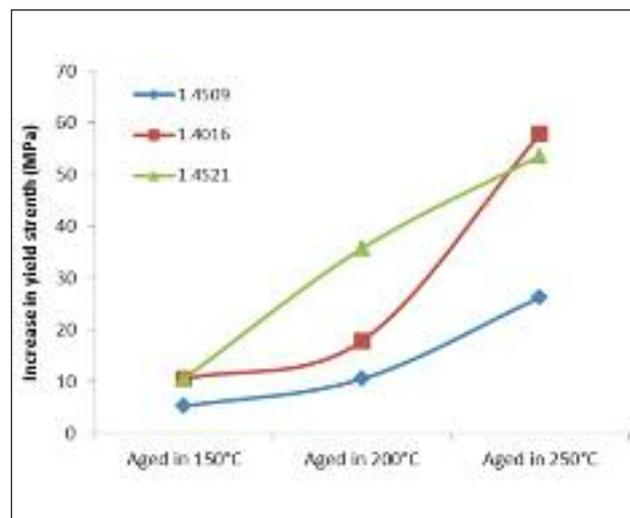
**FIG. 6** Increase in yield strength due to aging treatment.
