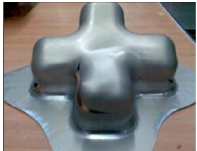
FIG. 3 Photograph of the cross die part. This tool was used for deep drawing experiments at more complex forming states. For characterizing the tribology, both, the maximum draw depth at a fixed blank holder force and the draw force are measured.
