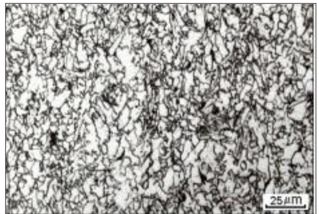
FIG. 14 Optical micrograph of a HSLA steel hot band. Etched with 2% Nital. (35,37)
