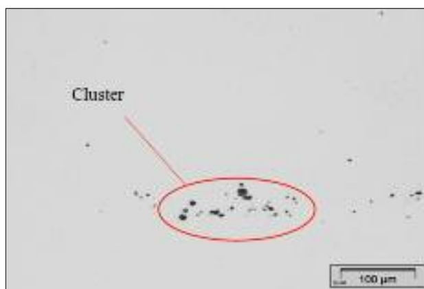
FIG. 1 Poor macro-cleanliness by clustering of alumina particles [3].
