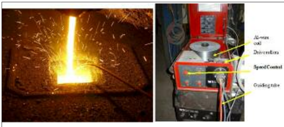
FIG. 6 Left: Billet mould with open pouring melt stream and guiding tube for Al-wire; right: Al-wire feeding device.
