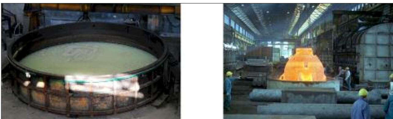
FIG. 6 Vasche di spegnimento mediante polimero in Area Fucinataura. Quench tanks with polymer in the Forging Department.
