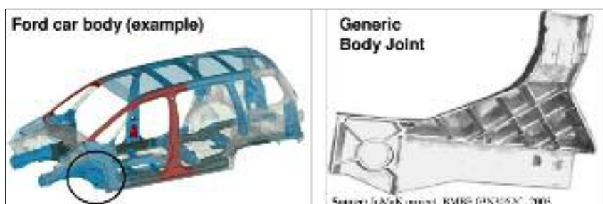
FIG. 13 Generic Body Joint produced by FORD.
