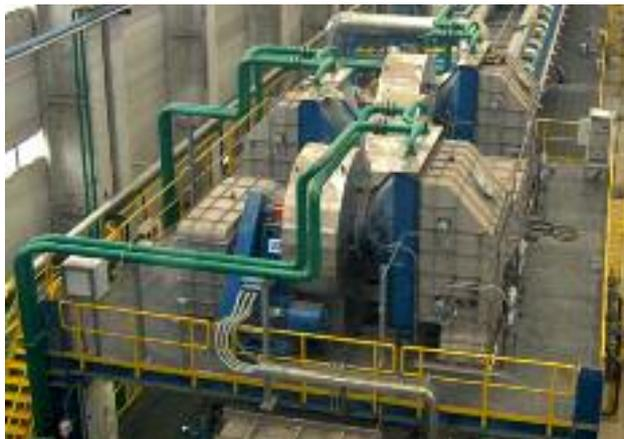
**FIG. 7** Compact design for horizontal jet cooling.
