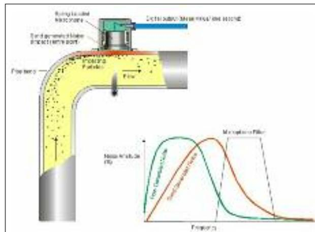
**FIG. 2** *Non-intrusive acoustic sensors, principle of measurement.*
