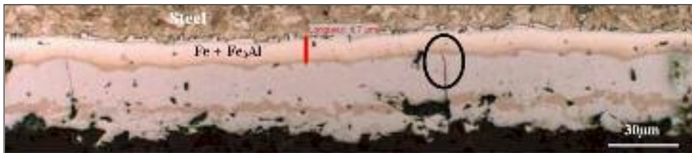
FIG. 8 Al-Si coating microstructure after press-hardening.
