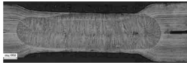
Fig. 7 - RSW welding spot between TWIP steel sheets. Axial metallographic section. Light microscope.
