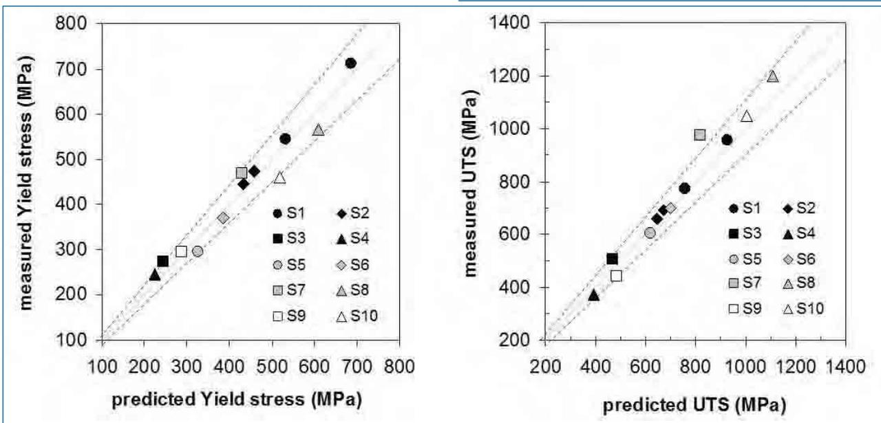
**Fig. 6 - Comparison between the experimental ultimate strength (UTS) and the yield stress (0.2) and the calculated ones by the model.**
