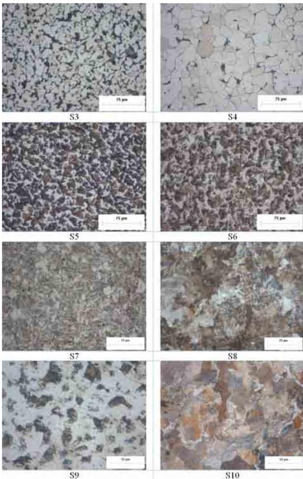
**Fig. 4 - Microstructure of the steels obtained by OM.**
