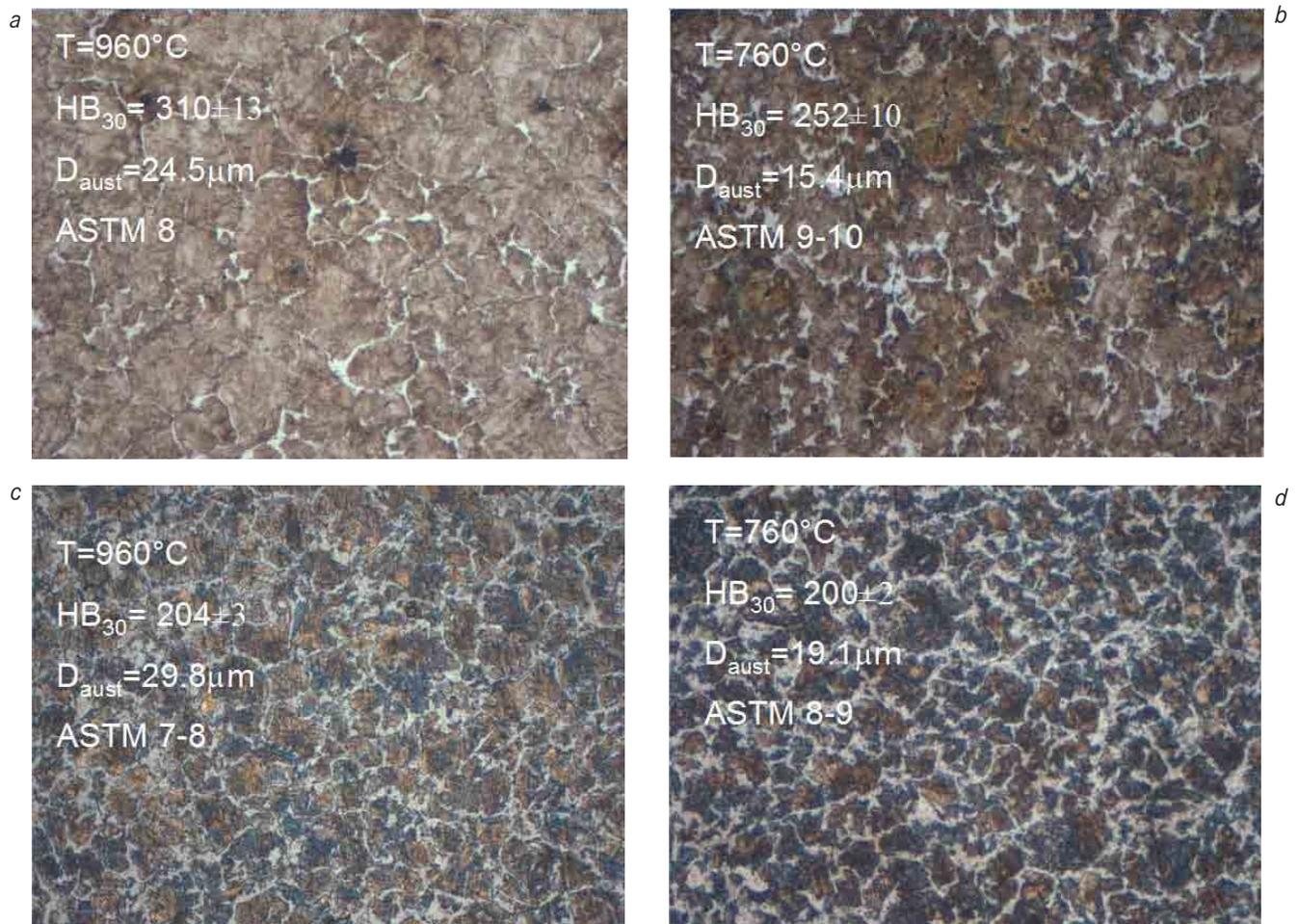
**Fig. 3 - Microstructure of steel S1 (a,b) and S2 (c,d) rolled at 960°C and 760°C.**
