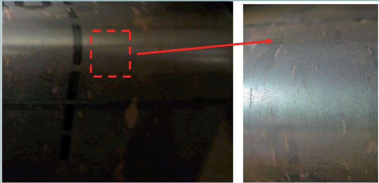
**Fig. 7 - Shape and surface quality of banded 1100MPa grade strip steel, bending line in transverse direction relative to the rolling direction ( $R=2.3t$ ).**
