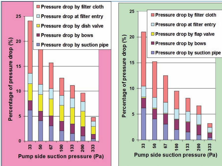
**Fig. 7 - Pressure drop by various structural elements between pump set and metallurgical vessel and the influence of pressure (Q=100000 m<sup>3</sup>/h, DN1000. L=100 m, 6x90° bows, 400m<sup>2</sup> filter, dish valve pink left, flap valve green right)**
