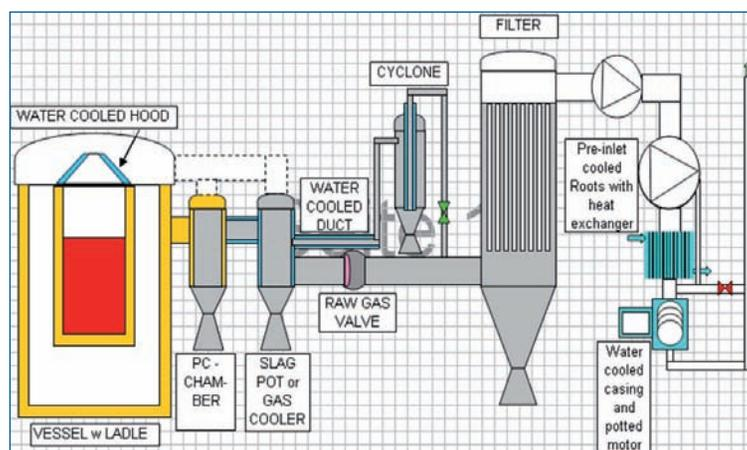
**Fig. 4 - Sketch of a universal off-gas preparation line showing the various possible elements for post-combustion, gas cooling and dust abatement.**
