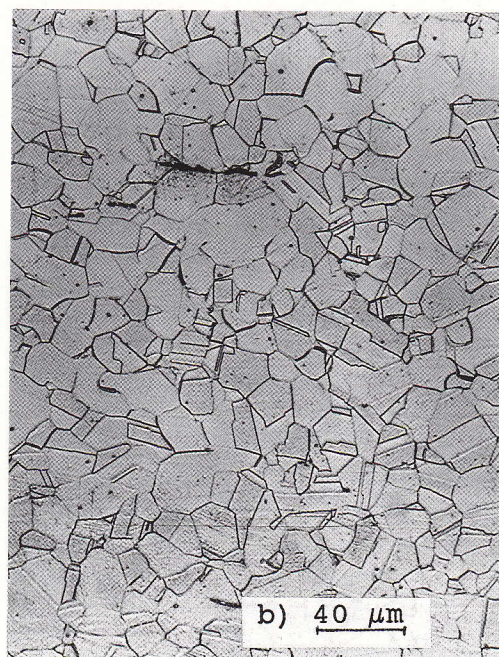
b) deformed at 1000°C, 5 s -1 showing refined DRX grains.
