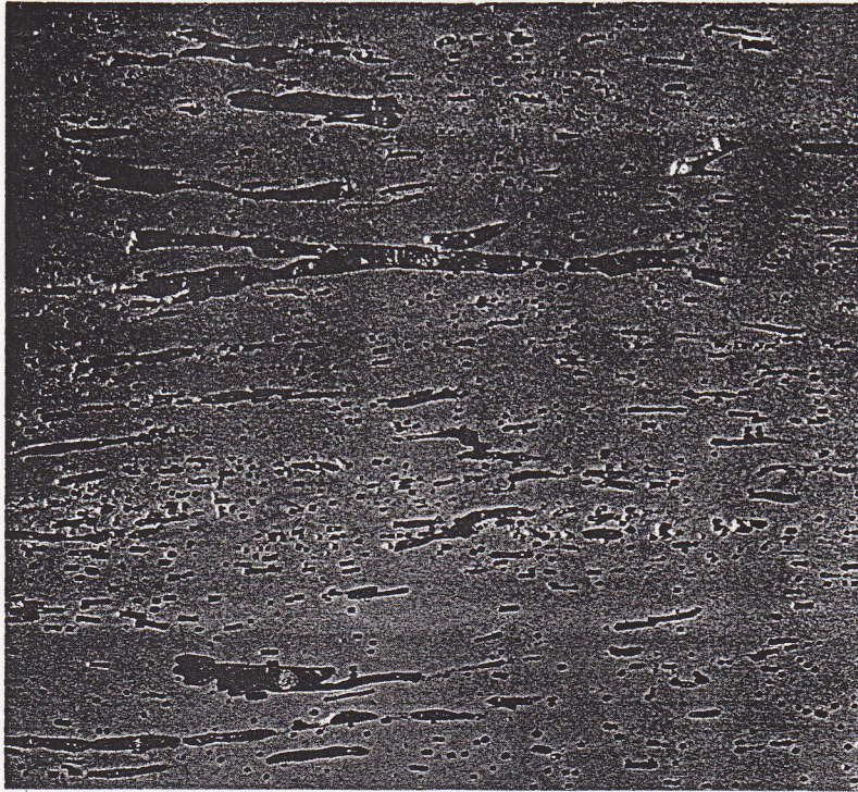
Fig. 5 (a): a) Microstructure of nonmetallic inclusions ( \times 100 )
