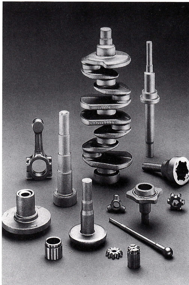
Fig. 1 - Hot forged automotive components.
